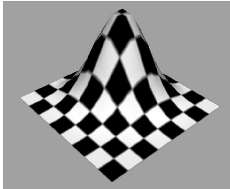
Figure #17: Uneven UV distribution for NURBS surface
