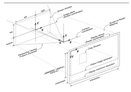
Figure 4.1: Camera-to-Raster Projection Geometry
