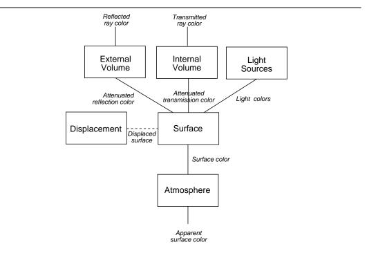
Figure 9.2: Shader evaluation pipeline
