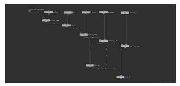
Figure 5.3: A screen-shot of the FLIP Liquid configure objects interior network in Houdini. Data is piped in via the top-left most node. Nodes at the top are field visualisers, and nodes at the bottom are our scalar and vector fields to be visualised.
