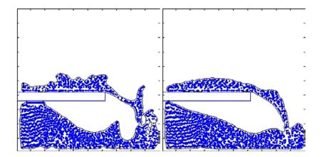
Figure 2.1: A comparison between the results of the FLIP and PIC methods for the same simulation. Image taken from Zhu and Bridson (2005).
