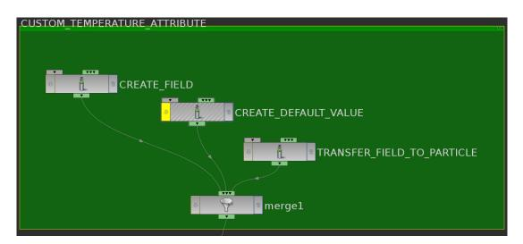
Figure 7.3: We create and initialise FLIP liquid temperature attribute.
