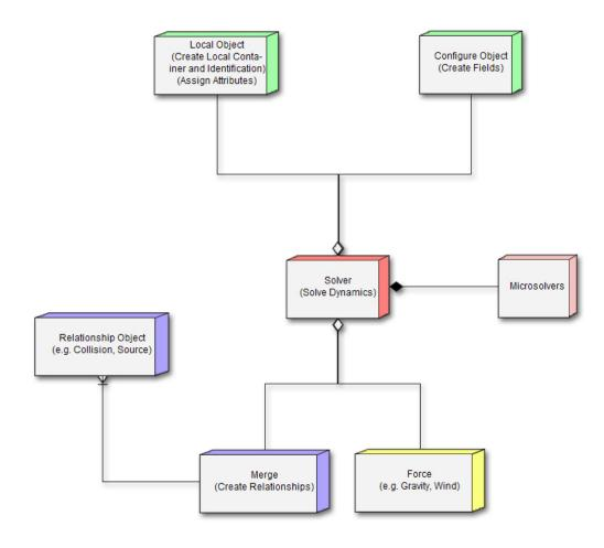
Figure 5.1: An overview of the DOP Network necessary for our FLIP Pyro solver.
