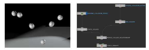
Figure 5.4: A RBD ball bounding on a ground surface. The merge node creates the collision relationship between the ball and the ground objects.
