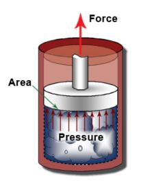
**Figure 3.2:** Pressure = Force per unit of area. Lowering the piston increases pressure, and vice versa. Image taken from Baratuci (2006).
