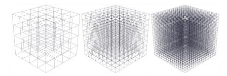
**Figure 3.4:** Three Eulerian grids, with resolutions of  $4^3$ ,  $8^3$  and  $16^3$  respectively. Note that doubling the resolution increases details eight fold each time.
