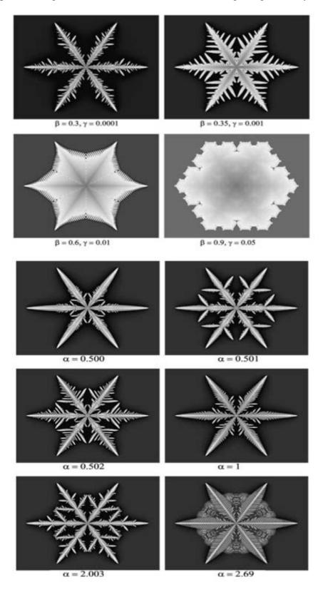
The variables of the diffusion constant for Beta =0.4 and Gamma =0.0001 It demonstrates that for Alpha = 0.5, 0.501, 0.502 give very different crystallised structures. One thing they all share is that they all exhibit dendrite growth.
