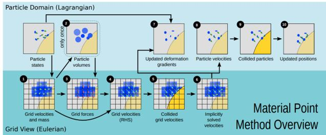
The particle-based representation of the material allows for a way to simply deform the material without causing mesh entanglement and the representation through particles allows splitting and merging of objects with different materials and behaviours. This makes it an appropriate method for simulations like melting. The Material Point Method Consists of 10 steps:
