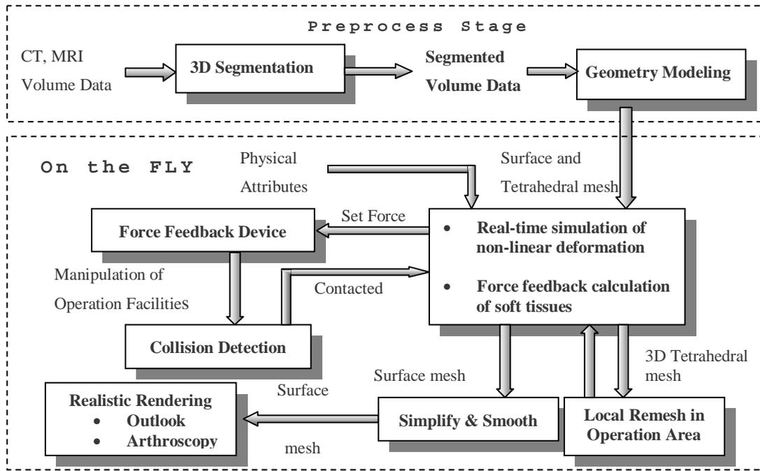
Fig 1 The system architecture of the virtual arthroscopy training system
