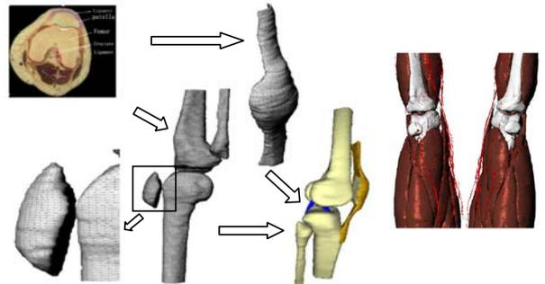
Fig 2 The procedure of mesh generation on the base of 2D medical images
