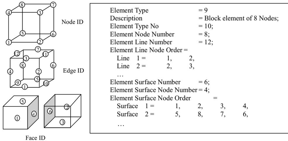
Fig. 2. Element set data structure.
