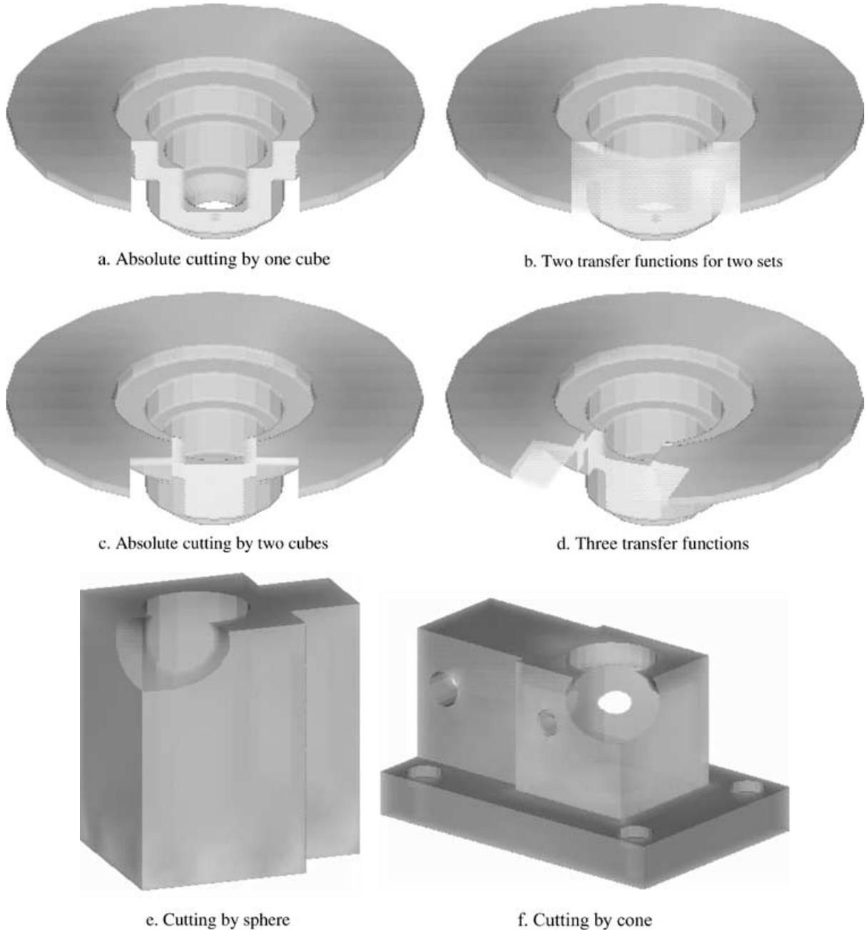
**Fig. 16.** Example of volume cutting by convex polyhedra.
