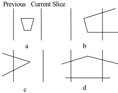
**Fig. 7.** Relative position between facet and two adjacent slices.
