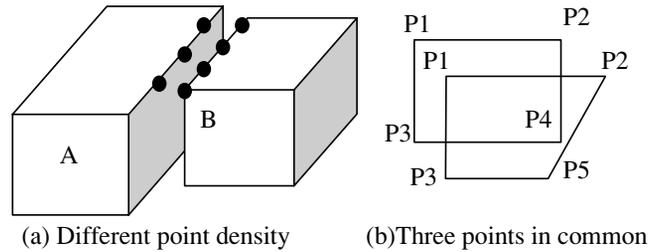
Fig. 5. Three nodes do not determine a common face.
