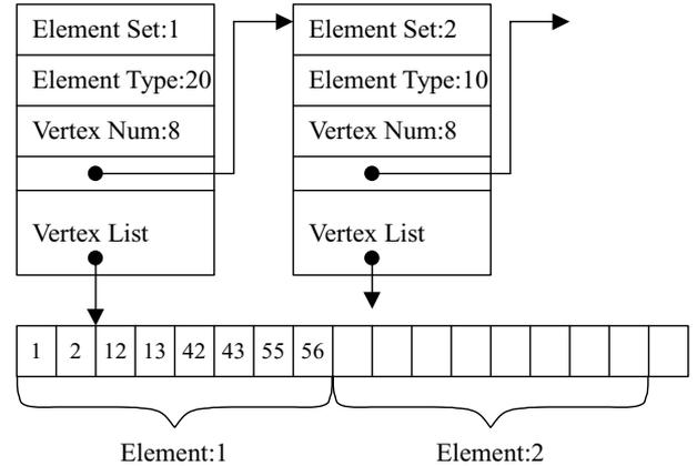
Fig. 1. Element set data structure.
