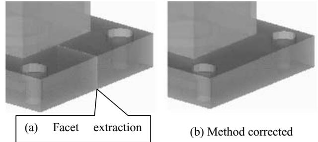
Fig. 4. Example of out-faced facet extraction.
