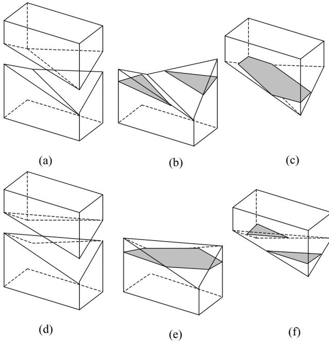
**Fig. 9.** Sliced polygon forming in case of concave element face.
