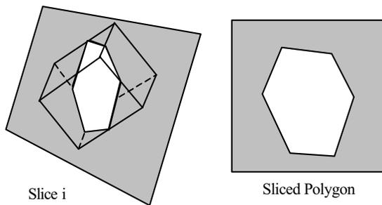
**Fig. 11.** The sliced polygon between the element and slices.
