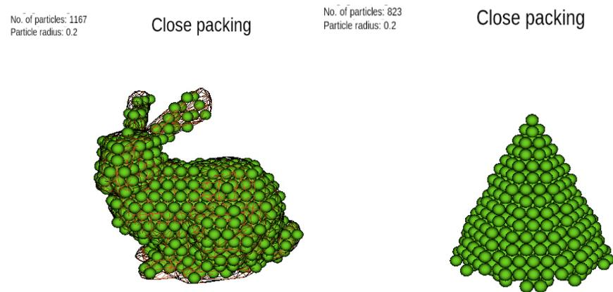
Figure 5: Hexagonal close packing
