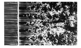
Figure 2.1: A uniform laminar stream of smoke passing through a perforated plate. Instability of the shear layers leads to turbulent flow downstream. Photograph taken from (Van Dyke, 1988).
