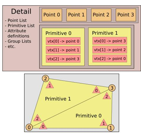
Figure 3.8: Geometry Structure in Houdini (SideFX 2011b)
