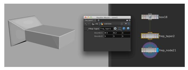
Figure 4.11: Example of the taper node
