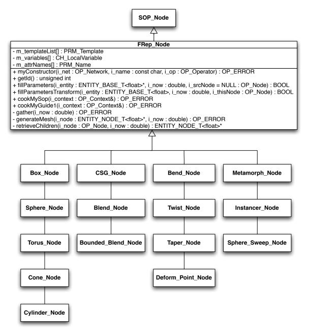
Figure 4.1: Class diagram of custom Houdini nodes
