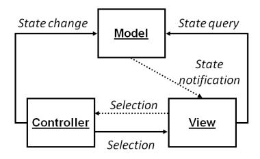
Figure 3.4: A Model-View-Controller diagram: The general design pattern (Kravtsov 2011)
