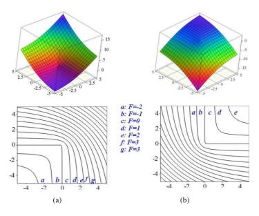
**Figure 2.2:** Set-theoretic operations based on R-functions: (a) Union and (b) Intersection (Kravtsov 2011)
