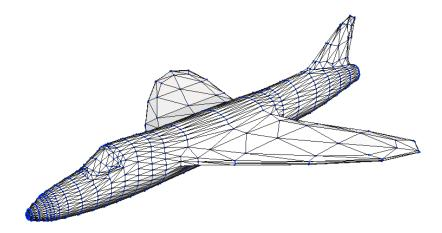
Figure 2.1: Example of a boundary representation: triangle mesh model
