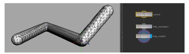
Figure 4.13: Sphere sweep node using a standard Houdini curve as input
