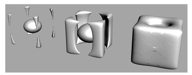
Figure 4.14: Offset node using different offset values: -0.5 (left), 0 (middle), 0.5 (right)
