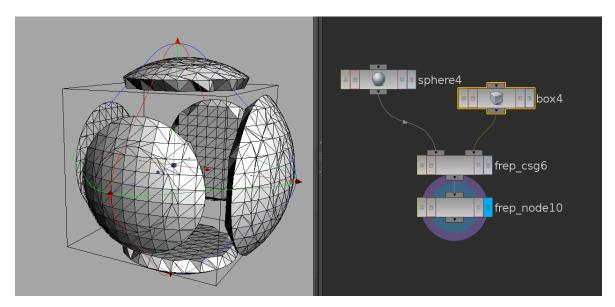
Figure 4.8: Example of a CSG node used to perform a subtract operation
