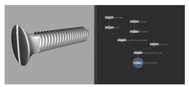
Figure 5.1: Screw model with its corresponding node network and optimisation for sharp features
