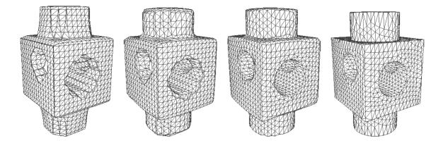
Figure 2.4: The leftmost and rightmost images demonstrate the initial and final triangle surfaces, before and after optimisation. The two middle images show intermediate stages. (Ohtake et al. 2002)
