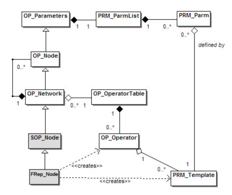
Figure 3.6: Basic class diagram for custom Houdini nodes (adapted from SideFX (2011a))
