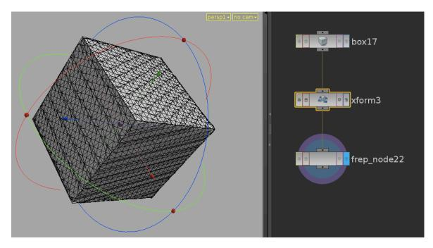
Figure 4.6: Transform node for scale, translation and rotation
