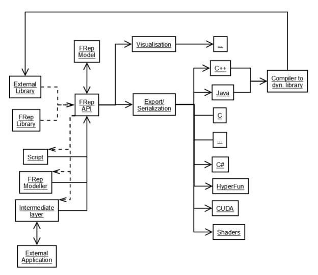
Figure 3.1: Full structure of the modelling environment and basic tools for FRep modelling (Kravtsov 2011)
