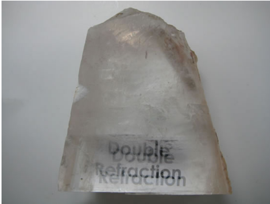
Figure 6 : Transparent calcite showing double refraction [GE]
