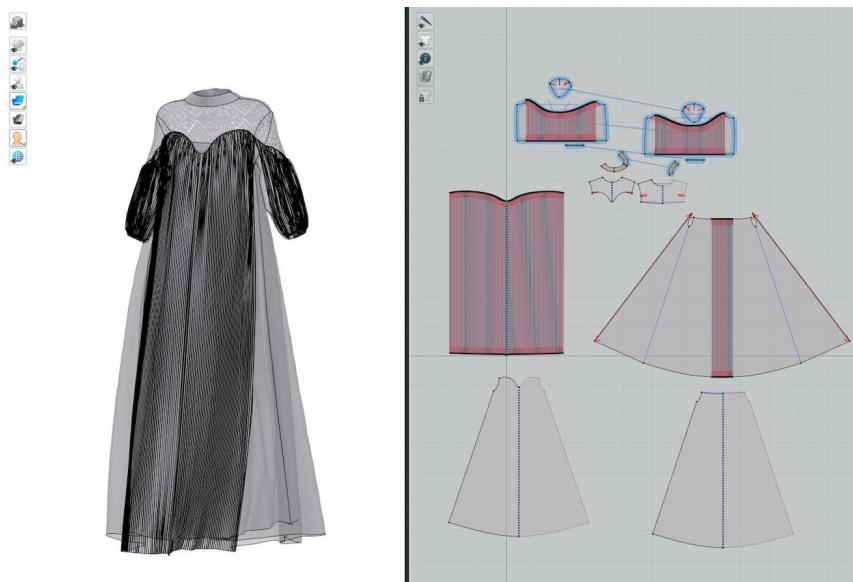
FIGURE 1.1: Example DCC tool overview including the 2D editor and 3D simulation view.
