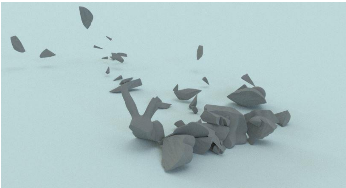
Fig 18: Result of surface based scattering for concrete
