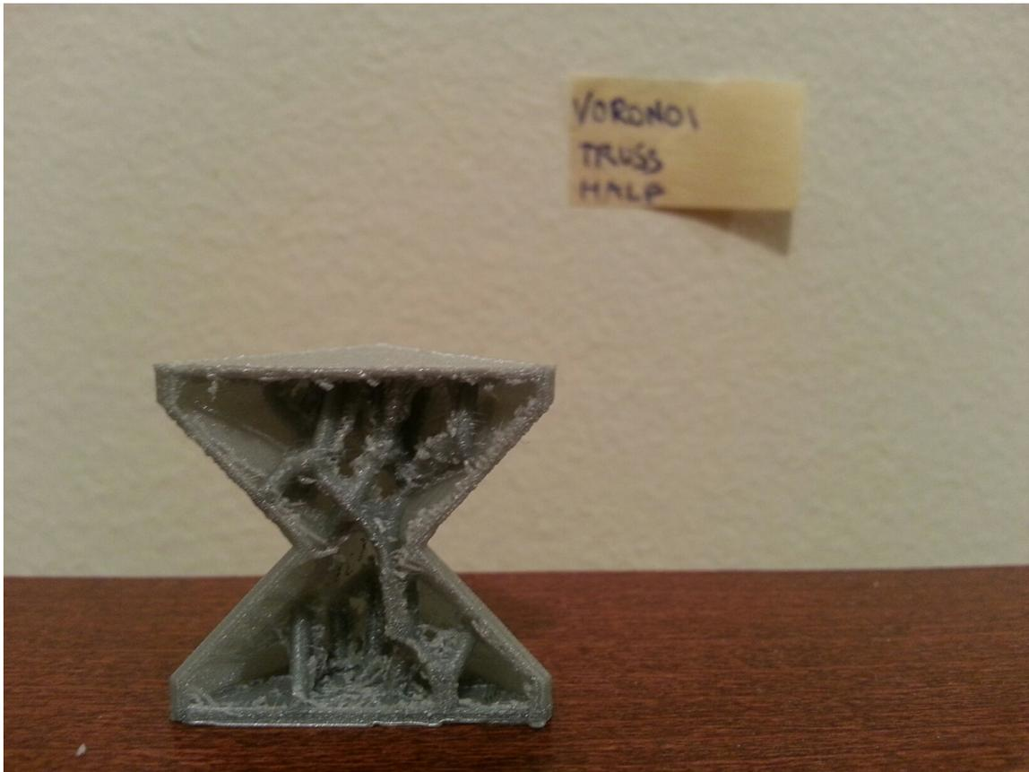
**Figure 6.3.2.1:** *Voronoi truss method cross section.*
