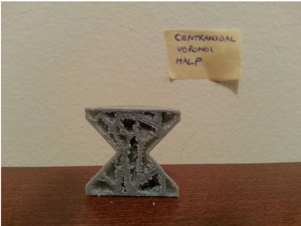
**Figure 6.3.1.1:** *A cross section of the centroidal voronoi method.*
