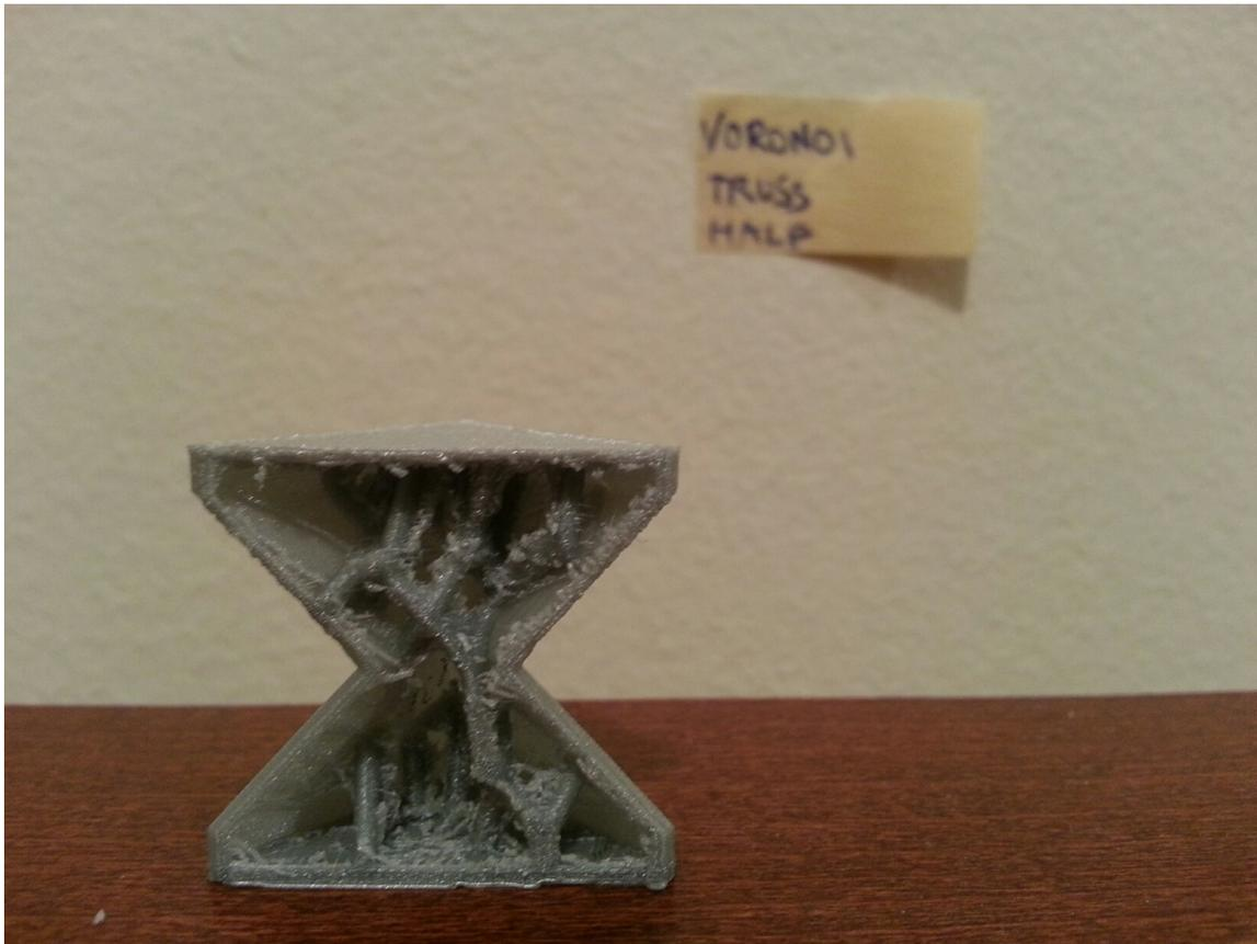
**Figure 6.3.2.1:** *Voronoi truss method cross section.*
