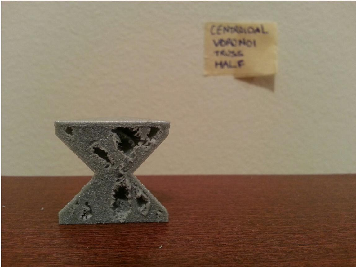
**Figure 6.1.4.6:** *Hybrid centroidal voronoi truss method cross section.*
