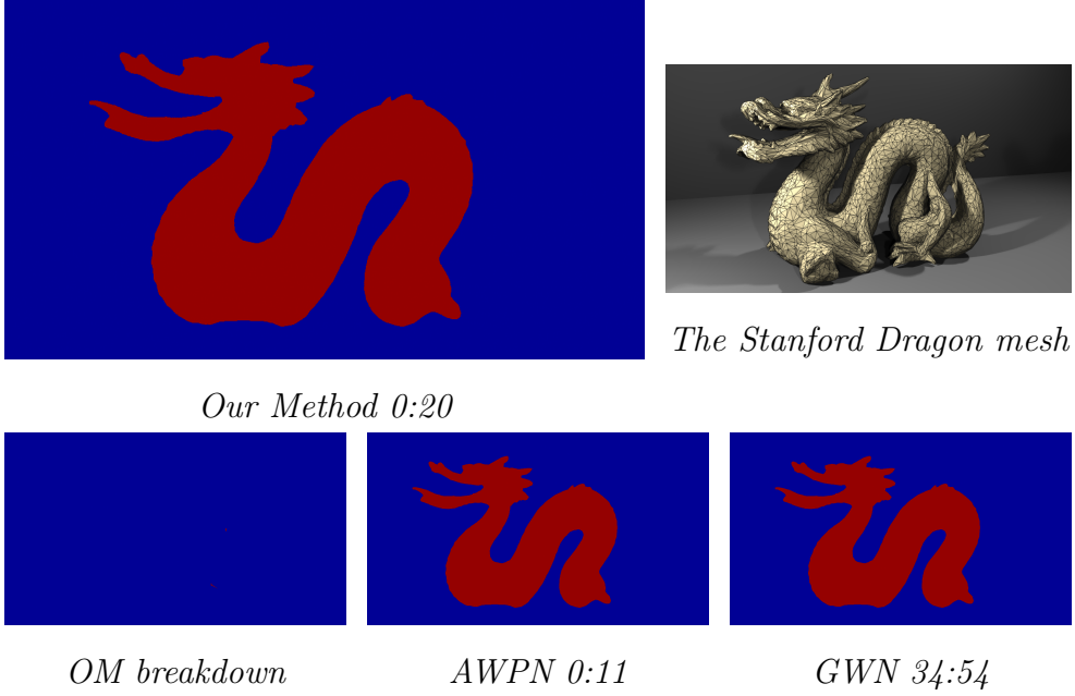
Figure 5.2: Classification of a plane through the Stanford Dragon containing 12500 faces and 8 self intersecting triangles. Model available from the Stanford University Computer Graphics Laboratory (2013)
