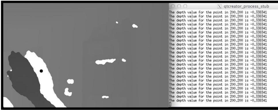
Figure 55: Depth returned from white noise. The dot is the point (200,200).
