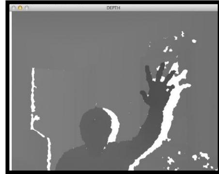
Figure 9: The raw depth stream from the Kinect.
