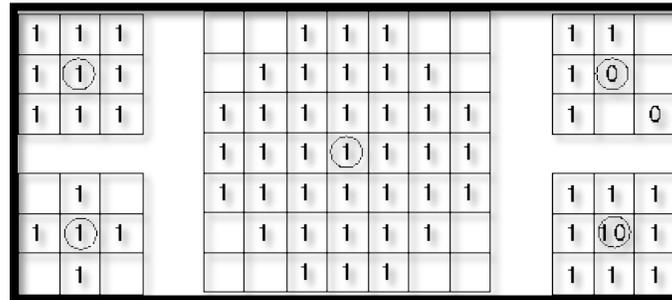
Figure 30: Different structuring elements of various sizes.
