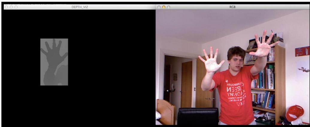
**Figure 58: The right hand is NOT affecting the detections. Only left hand is seen.**
