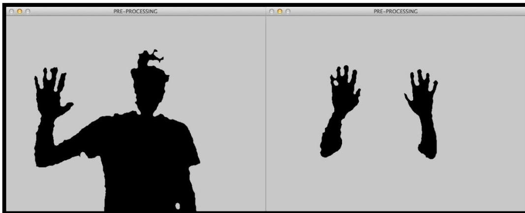
Figure 20: Binary threshold on the image matrix.
