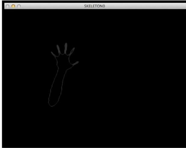
**Figure 32: The hand mesh after thinning.**
