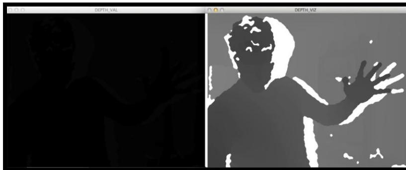
Figure 52: The 16-bit depth Values is on the left and the 8-bit depth Visuals are on the right.
