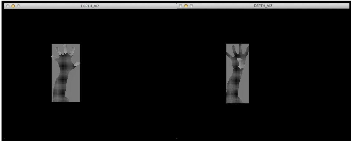
**Figure 66: Self-Occluded grid points.**
