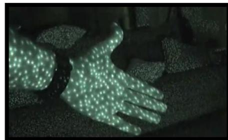
Figure 8: The Infra Red grid projection.
