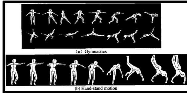
**Figure 2: 2D skeleton extraction using FCC.**
