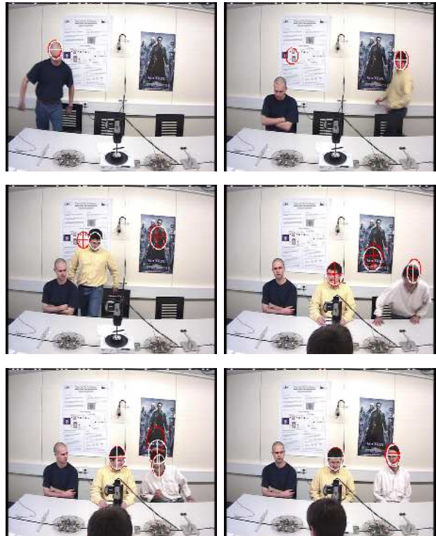
Figure 6: Frames 10400, 10500, 10550, 11070, 11090 and 11300 of Scenario C seen by Camera 2. Here the SIR tracker loses person 1 and later tracks person 3 with two ellipses simultaneously.
