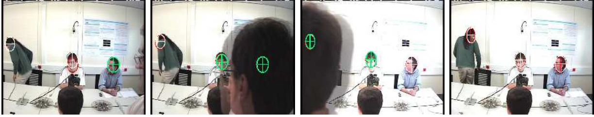
Figure 2: Occlusion handling. Frames 17125, 17130, 17135 and 17140 of Scenario C viewed from Camera 1. Suspended tracks are shown as green ellipses. (The halo effect around the occluding head is due to interlacing.)
