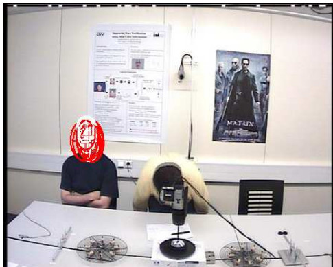
Figure 11: Head estimates at frame 10571 of Scenario C after 20 different runs of ICondensation starting from the first frame of the sequence. For each run, a red ellipse denotes the mean for the tracker initialised on the left-most person and the white ellipse the mean for the tracker initialised on the other person.
