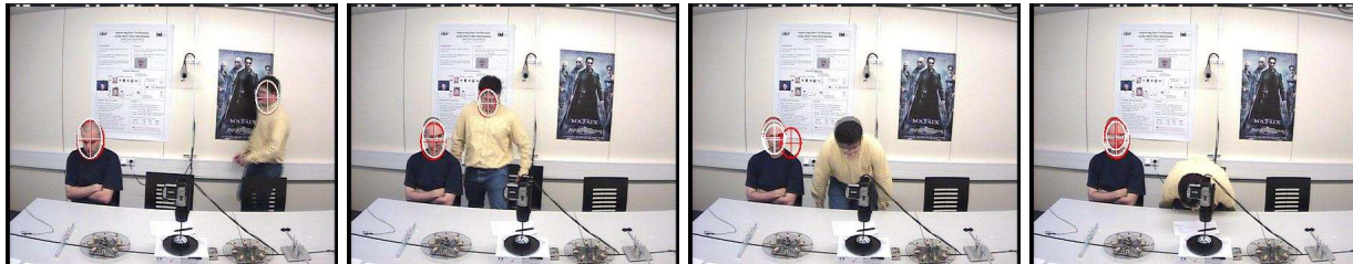
Figure 9: An ICCondensation tracker locking on to the wrong person. An unusual head pose resulted in a poor importance function causing the tracker to jump to another person rather than track through this temporary change in color distribution.
