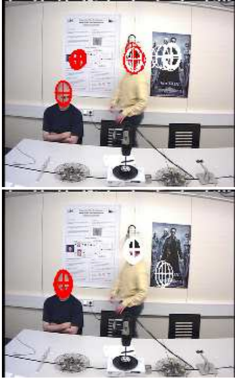
Figure 7: Head estimates at frame 10520 of Scenario C after 50 different runs of the tracking algorithm starting from the first frame of the sequence. The upper image shows the results using SIR and the lower image the results using ILW. Each ellipse is the mean of the ten strongest particles.
